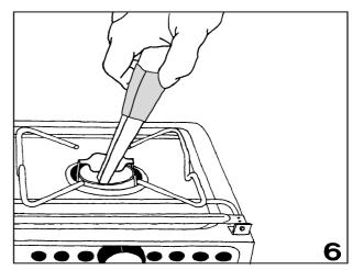
NOTE: If stove is warm from previous use, burner may ignite, then immediately go out. In this event, blow down into the burner opening to dissipate vapor and relight as above.
