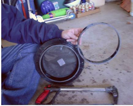
After sawing, you will want to sand the edge smooth, using increasingly finer grits of sandpaper until edge is smooth.
