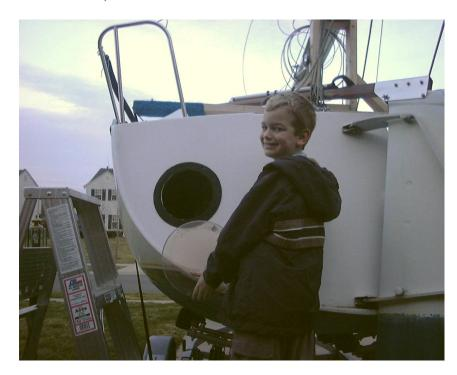
Remove all existing gasket material with scraper and adhesive remover, being careful not to scratch gelcoat.
