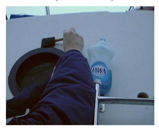
Remove trim ring and place wide bead (about 1/4") of silicone in circle around opening, in gap between opening and port, and in every open hole whether from original port or your drilling through. Place and squeeze trim ring up against silicone bead. A small amount of excess silicone will appear from edge of ring.
