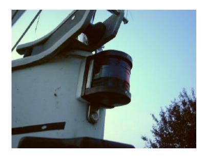
Drill two mounting holes with 1/8" drill bit, and one 3/16 (maybe slightly bigger) for wire.
