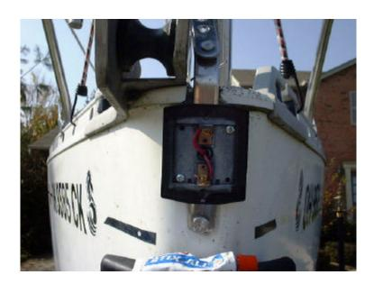
Replace light bulb and cover, and tighten cover screws.
