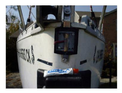
Remove light bulb. Strip and pass one wire (makes no difference) through top terminal screw and the other through the bottom.
