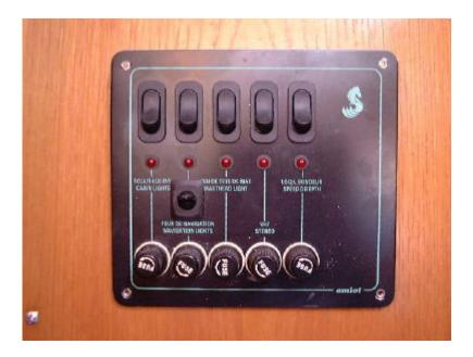
I then cut the existing line from the fuse holder that ran to the bus about an inch from the fuse holder (just long enough to barely reach the center terminal), and soldered the short end to center of switch and other to bottom terminal. This would be so that when switch is up, Nav lights on Mast would be on. Next I crimped and soldered a lug to the black wire and added it to the grounding block. I then soldered the remaining red wire to the upper terminal on the switch.
