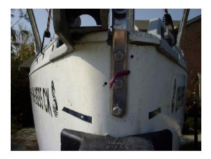
Pass wire through light mount. Apply silicone to holes, and backs of standoffs. Screw with #8 screws into place. Notice tube of Elmer's Stix All Silicone. Ideal size.
